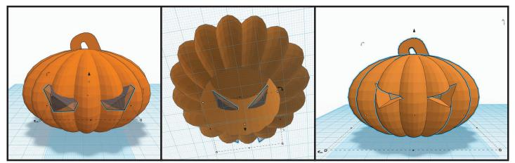
• Cut the eyes from the pumpkin. To do this, click to select the first eye, hold shift and click the second eye. In the inspector window near the top right, change the eyes to "Hole". Draw a selection box over both the eyes and the pumpkin. In the top right tool bar, click "Group".
