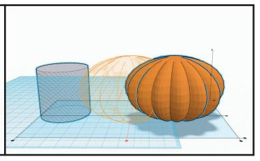
• Create selection box over both the pumpkin and the cylinder. In the top right tool bar click "Adjust" > "Align...". Click the front middle line + circle to center and the side middle line + circle to center. With both objects still selected, in the top right tool bar click "Group".
