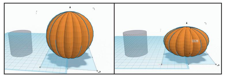
• Click on the pumpkin to select, using the tiny white box on the top middle, click + drag height to "50.00mm".
