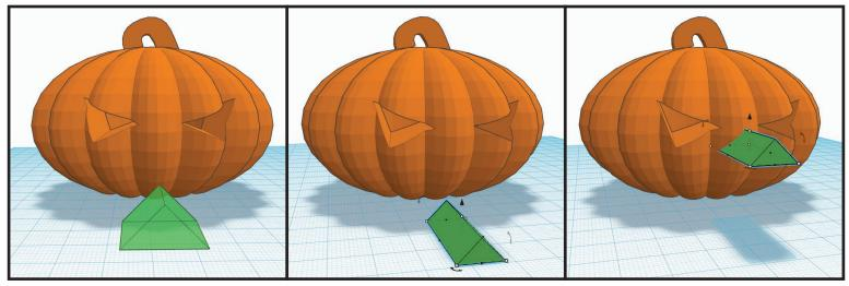
• Click in the center of the Roof/Wedge object and drag to position on the pumpkin. Use the black arrow at the top middle to move higher/lower on the pumpkin. Also use the rotation arc on the floor plane to rotate as needed.
