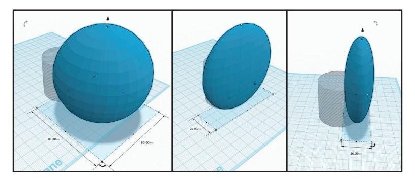
• Click on squished sphere to select, press "CTRL+C" to copy and "CTRL+V" to paste. With the new squished sphere still selected, click + drag the rotate arc on the floor plane one snap on the inside degree circle.
