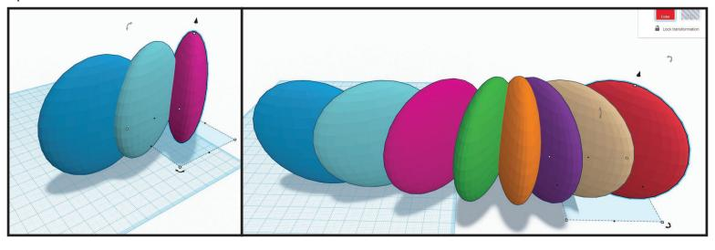
• Create a selection box over all of the squished spheres in the workspace to select. In the top right tool bar click "Adjust" > "Align...". Click the front middle line + circle to center and the side middle line + circle to center. With all squished spheres still selected, in the top right tool bar click "Group".
